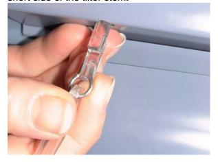
**10.** Locate the hole at the top of the long groove on the tilter stem and insert the wand connector clip.
