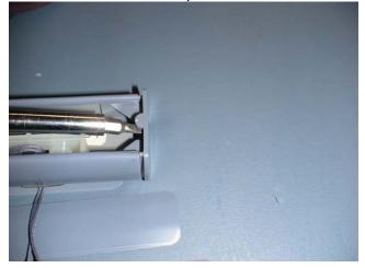
**4.** Slide the tilt rod out the opposite end of the tilter until it is free of the tilter.
