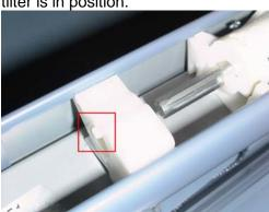
7. Slide the tilt rod back into the tilter.
