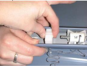
**6.** Place the new wand tilter into the rail, guiding the stem through the cut out. Be sure the tab is to the top. Push down firmly on the back side until the tilter is in position.
